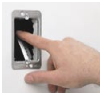
Low-voltage mounting bracket: For installing wall plates or ZIM-4 input modules. Cut a hole in the drywall, bend the metal tabs behind the wall, then lock the tabs in place with screws. Then attach the wall plate or ZIM-4 to the bracket.
