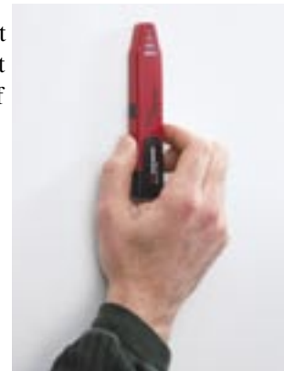
Stud sensor: Indispensable tool for finding the right places to mount speakers, wall plates and controls.
